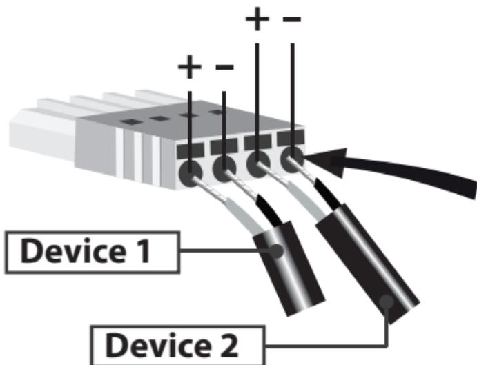
Twist the bare wire together and trim it with a cutting tool so that when it is inserted into the plug it is not exposed and does not cause bad contact with other cables.
