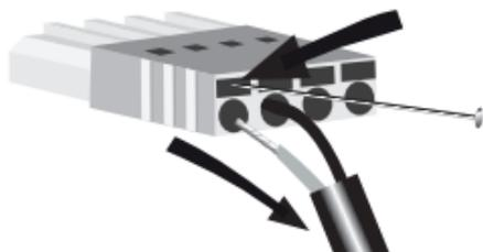
Next, carry out the same procedure on your sensors (INPUTS). Keep in mind that inverting the polarity of the sensor you will also invert the data recorded by TankBot. You can invert this polarity on the software without the need to re-wire the system.
