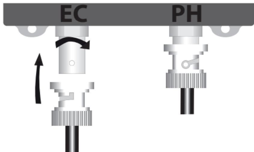
**Never exchange the position of the pH and EC sensors.**
