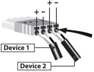
Twist the bare wire together and trimm it with a cutting tool so that when it is inserted into the plug it is not exposed and does not cause bad contact with other cables.
