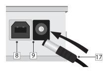
With this connection made your module is powered and the LED indicator (13) should start to blink. You also now have power available on the Power output connector (1).
