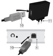
Connect the transformer (11) to a 110~230V<sub>AC</sub>/5V<sub>DC</sub> power outlet.
