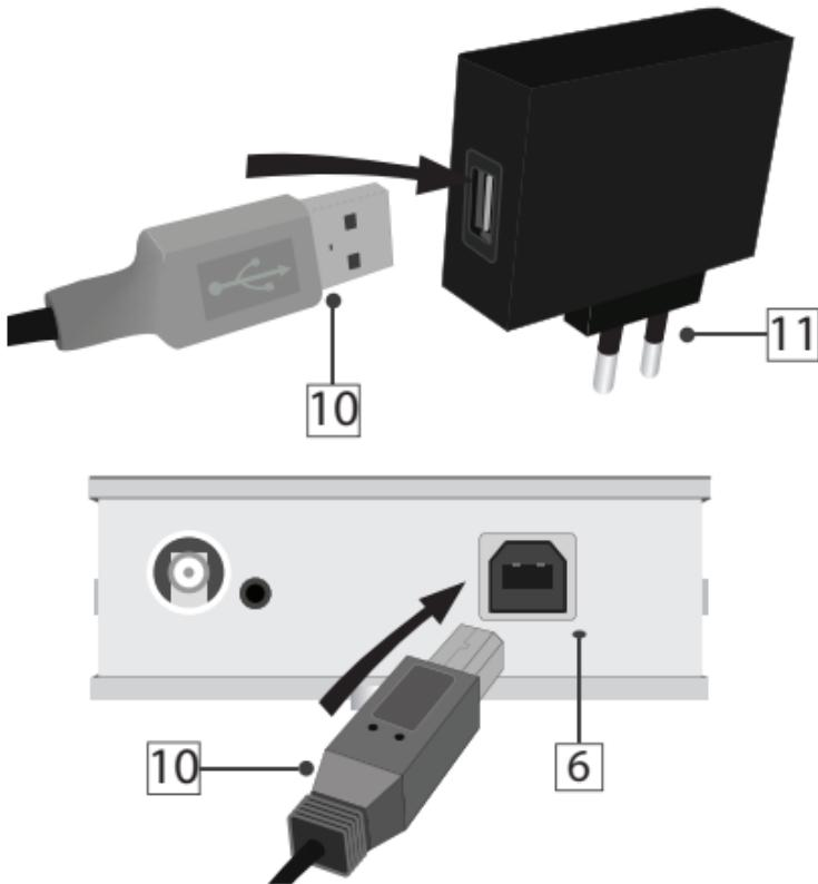
Connect the transformer (11) to a 110~230V<sub>AC</sub>/5V<sub>DC</sub> power outlet.
