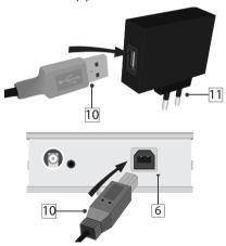
Connect the transformer (11) to a 110~230VAc/5VDC power outlet.
