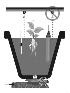
The moisture sensors for substrate and flood detectors have resistive technology and are vulnerable to corrosion caused by electrolysis.
