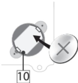
Place the battery cover (15) on the battery holder (10) then insert the screws (16) without exceeding its tightening.
