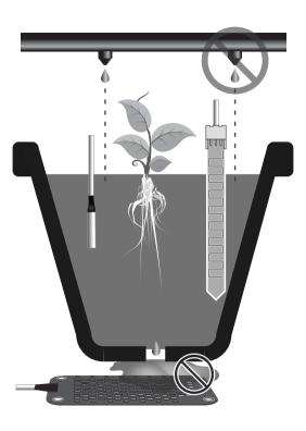
The moisture sensors for substrate and flood detectors have resistive technology and are vulnerable to corrosion caused by electrolysis.
