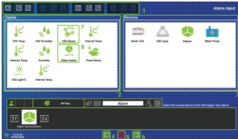
Figure 10-3 – Alarm Input condition configuration
